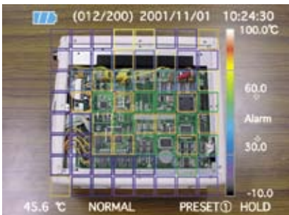
■ Detection of Heating in Circuit Boards and Electrical Devices
